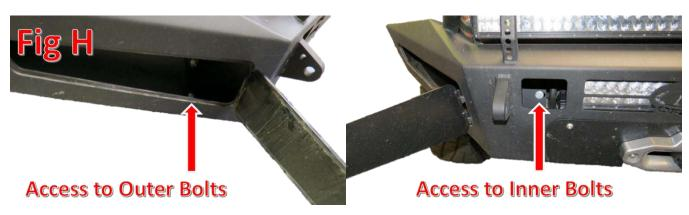
5. Align the bumper so that it sits straight in relation to the bottom of grill, headlights, and front fender flares. Tighten the bumper mounting bolts to 70 foot pounds. A second person will come in handy for this step as well.
