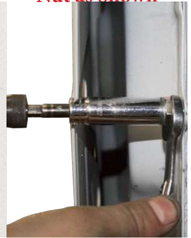
Tighten Rivet Nut as Shown
