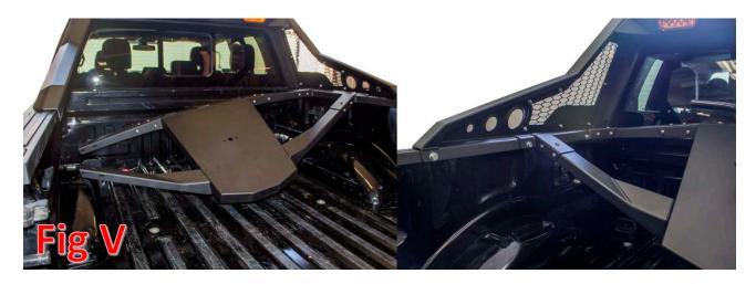
4. Set the roof rack section in place. Then, use the supplied 3/8" Bolts (x16), 3/8" Washers (x16), and 3/8" Nuts (x16) to loosely secure it. The bolt holes can be accessed through the toolbox openings (The picture does not show all of the mounting bolts). Once all mounting bolts have been installed, torque them to 20 foot pounds. (Fig W)
