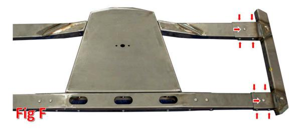
4. Install the receiving end of the tire spinner using the supplied 3/8" Bolts (x2), 3/8" Washers (x2), and 3/8" Nuts (x2). (Fig G) Tighten these bolts to 20 foot pounds.
