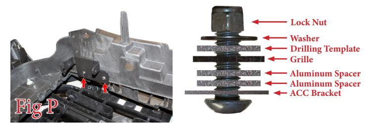
18. Set the rest of the bracket and module in place. Use the supplied Black 1/4" Bolts (x4), Black 1/4" Washers (x4) and Black 1/4" Lock Nuts (x4) as well as the supplied 1/4" Carriage Bolt (x1), 1/4" Washer (x1) and 1/4" Lock Nut (x1). (Fig Q) Make sure to adjust the tilt on your Adaptive Cruise Module so that the module is parallel to the front face of the grille, and perpendicular to the ground.
