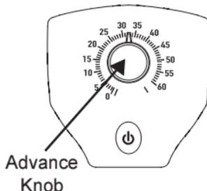
3. **View timing marks. Loosen distributor hold down bolt and turn distributor until moving mark is aligned with stationary “0” degree mark.**
