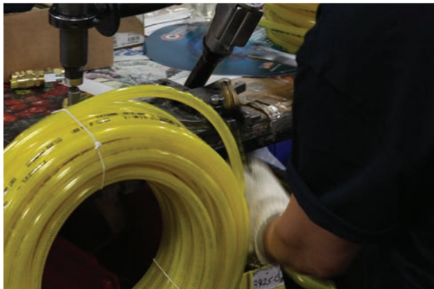
(Left) Installing fittings to Flexeel in our factory in New Jersey.
