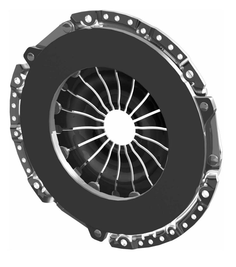
**Faults/Symptoms:** Symptoms include: clutch chatter/shudder, slipping clutch, abnormal odor, low pedal clutch take-up. Faults include: worn or damaged friction material, broken or damaged damper springs, oil contamination,
