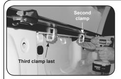
C. Next install a 2nd clamp at midway point of box and rail. Now check rail for level. *See photo at left and illustration below.* If rail tilts up, move clamps down and tighten. If rail tilts down, move clamps up and tighten.
