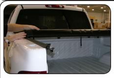
A. Unroll cover and place rear bar into strikes on side rails and press down on bar to close (20-30 pounds pressure).
