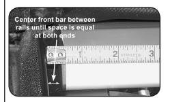
D. Center the front bar between the two side rails.
