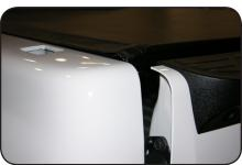
B. Close tailgate slowly - top of tailgate should fit snug under cover bar. If tailgate rubs bar too hard, raise rails by loosening rear clamps, adjust rails up and retighten clamps. If there is too much gap between tailgate and cover bar, lower rails by loosening rear clamps, adjust rails down and retighten clamps. Check cover tension by releasing trigger latch and open and close rear bar several times. It should snap down when closing.
