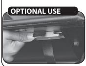
Manual Slide Lock (use is optional) is located under cover bar on passenger and driver side - push slide lock to engage, pull to disengage.
