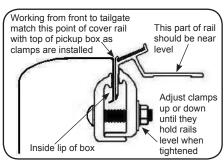
D. Install third clamp as close to tailgate as possible. *See photo*. Make sure all clamps are placed in best up or down position for a level rail. Then recheck all clamps to insure adequate tightness.
