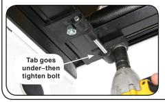
E. Then tighten bolt (left loose earlier) under front bar on each tension adjuster.
