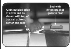
A. Align weatherstrip edge of side rail against inside lip of box and **push rail forward until it stops against front of box - nylon strike goes to rear.** See photo at left to determine how high up to mount rail.
