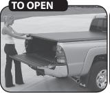
Open tailgate on driver side release trigger latch and lift up on rear of roll bar.
