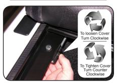
C. Cover fabric should sound drumlike when tapped on. If adjustment is needed, roll cover open and to loosen turn EZ-Dial Clockwise. To tighten turn EZ-Dial Counter Clockwise. Always turn Dials in Equal amounts. See photo at left.
