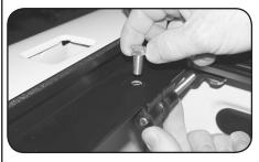
B. Slide left tension adjuster over until it engages under side rail. (See photo in Step 3 E for tension adjuster tab under side rail.) Push bar back and forth to line up holes-do not turn dial wheel. Insert bolt from top and nut from bottom.
