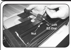
A. The cover comes pre-rolled to its normal open position for ease of installation. Set pre-rolled cover on tailgate with front bar facing up as shown. Align EZ-Dial Tension Adjuster (marked L) on driver side of cover - positioned as shown in photo at left.
