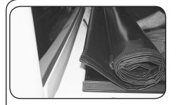
A. Set rolled up cover on rails at front of box (behind cab) with bar facing up. Roll cover bar onto front of rails and fold/tuck vinyl flap under. Now bar will face down. Let straps hang to inside of box. Push cover bar forward until it sets flat on front of side rails and overhangs them.
