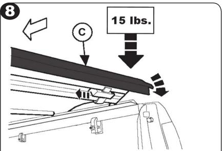
Check tailgate closing. Adjust rear of rails up for more tailgate clearance, or down for less clearance. Check cover tension with tailgate down. Closing bar down and latching should take about 15 lbs. of pressure.
