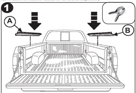
**Driver Side** - end of rail with slotted hole goes to front behind cab, trigger latch to rear.
