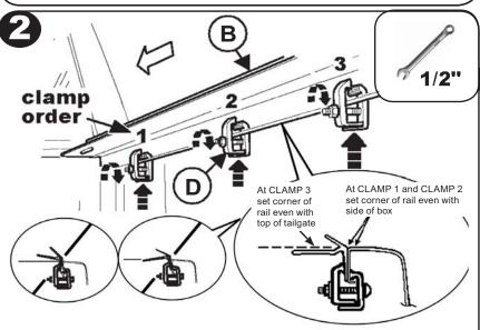
Position front and rear clamp about 8 inches from ends and one clamp in middle. Follow clamp order sequence in diagram. Clamps can be moved up or down for rail leveling adjustment.
