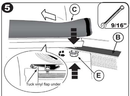
At each end, align nut in front bar with slotted hole on rail. Insert a bolt, flat and lock washer up through slotted hole and turn into nut. Center bar between rails. Then adjust bar until bolt is centered in slotted hole and tighten. Do same with bolt at other end.
