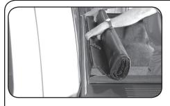
A. Set rolled up cover on rails at front of box (behind cab) with bar facing up. Roll cover bar onto front of side rails and fold/touch vinyl flap under. Now bar will face down. Let straps hang to inside of box. Push cover bar forward until it sets flat on front of side rails and overhangs them.
