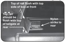
A. Align weatherstrip edge of side rail against inside lip of box **and push forward until it stops against front of box** (nylon strike goes to rear). At front, rail should be flush with top side of box. At rear, rail should be flush with top of tailgate.
