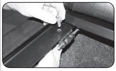
B. Slide left tension adjuster over until it engages under side rail. (See photo in Step 3 E for tension adjuster tab under side rail.) Push bar back and forth to line up holes-do not turn dial wheel. Insert bolt from top and nut from bottom.
