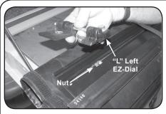
A. The cover comes pre-rolled to its normal open position for ease of installation. Set pre-rolled cover on tailgate with front bar facing up as shown. Align EZ-Dial Tension Adjuster (marked "L") on driver side of coverpositioned as shown in photo at left.
