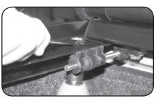
C. Hold bolt at top and tighten nut under side rail. Repeat procedure for right hand tension adjuster.
