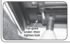
E. Then tighten bolt (left loose earlier) under front bar on each tension adjuster.
