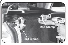
C. Install 2nd clamp on rail at midway point of box and rail. Check if rail is level. Install 3rd clamp as close to tailgate as possible. If rail tilts up, loosen clamp, lower it and tighten. If rail tilts down, loosen clamp, raise it and tighten.
