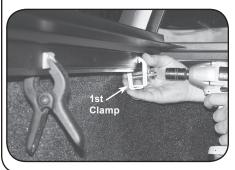
B. Hold rail in place with spring clamp and close tailgate to check height. Then place 1st clamp as close to front as possible and use ½" wrench to tighten.
