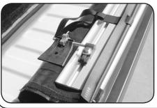
B. Turn 1-1/4" bolt with flat washer onto nut in bar. Leave loose for now. *See photo.* Repeat for XT-Dial (R) on passenger side of cover, and leave that bolt loose also.
