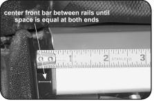
D. Center the front bar between the two side rails.
