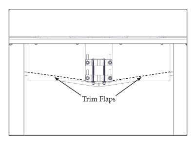
4. Trim bottom of flaps to match the angle of the frame (See Figure 4)
