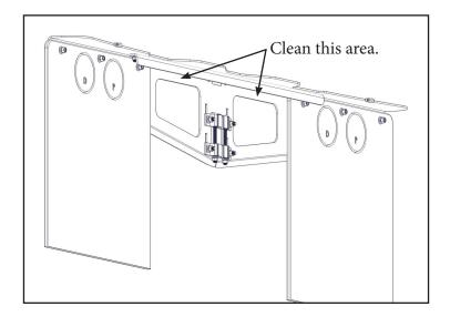
1. Use Alcohol wipe to clean backside of mud flap frame. NOTE: If adding flaps to an existing set of mud flaps, thoroughly clean backside of frame prior to using alcohol wipe.
