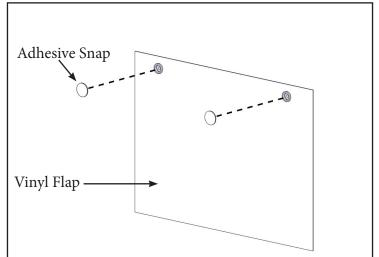
2. Attach adhesive snaps to vinyl flaps. Do not peel protective layer off now.
