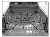
area of box (where seal adheres) with mild soapy water. Towel dry. Wipe with alcohol pad (save 2nd alcohol pad for later). See above.
