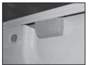
a) At front corner (behind cab) b) Hold up under box lip and c) Then push and compress foam d) Continue pushing foam into compress foam to fit inside lip.
