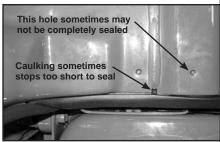
Sometimes hole is not sealed on floor and OEM caulking sometimes stops short at end of box. Seal with silicon if desired.
