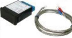
Digital temp. meter matches our Digital Volt & Amp meters. 20ft. remote temperature probe. Ideal for monitoring amps. Prevent overheating, which limit performance & distort sound quality. Perfect item to be used with our cooling fan controllers (FC-10 / FC-30). Face dimensions: 1 7/8" X 1". Cutout required: 1 3/4" x 7/8". Temp range 0-199°F
