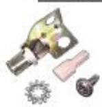
The fast, quick & cost-effective way to protect hoods and trucks without worrying about any switch alignment problems. Just screw the self-grounding body to hinge or lip portion of hood/truck with the TEK™ screw provided; adjust switch angle by bending bracket. (Switch only available MS2B)
