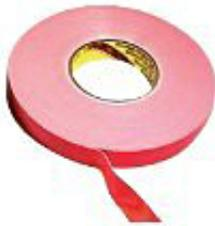
A closed cell foam tape coated on both sides with a pressure sensitive adhesive. It is well designed for attaching automotive trim molding, emblems and other articles where high internal strength is required. Size 1/2" x 20 yards.
