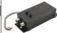
Converts any head unit output (low or high power, common or floating ground) to low level RCA outputs. Full D.C. isolation circuitry eliminates ground loops and engine whine. Adjustable right and left channel outputs (0-1 Volts). Will match up to any aftermarket amplifier. Input/output 4 or 8 ohm max. 25W.
