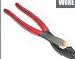
For insulated & non-insulated terminals & connectors. Thin nose permits work in confined space. Accommodates wire from No.10 to 22 AWG. Wire cutter in nose. Red plastic-dipped handles.
