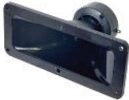
High output piezo horn. Frequency response: 2 - 24khz. Dimensions: 3 1/2" high, 7 5/16" wide, 4 1/4" deep
