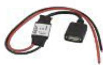
12 VDC In 5 Volt 2amp output to female mini USB
