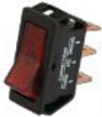
Two position that lights when on SPST. Switch and bezel are black. Specify lens color: RED, AMBER, BLUE or GREEN. Matching switch panel avail. Fits 7/16" x 1 1/8" panel cutouts. 12VDC light.
