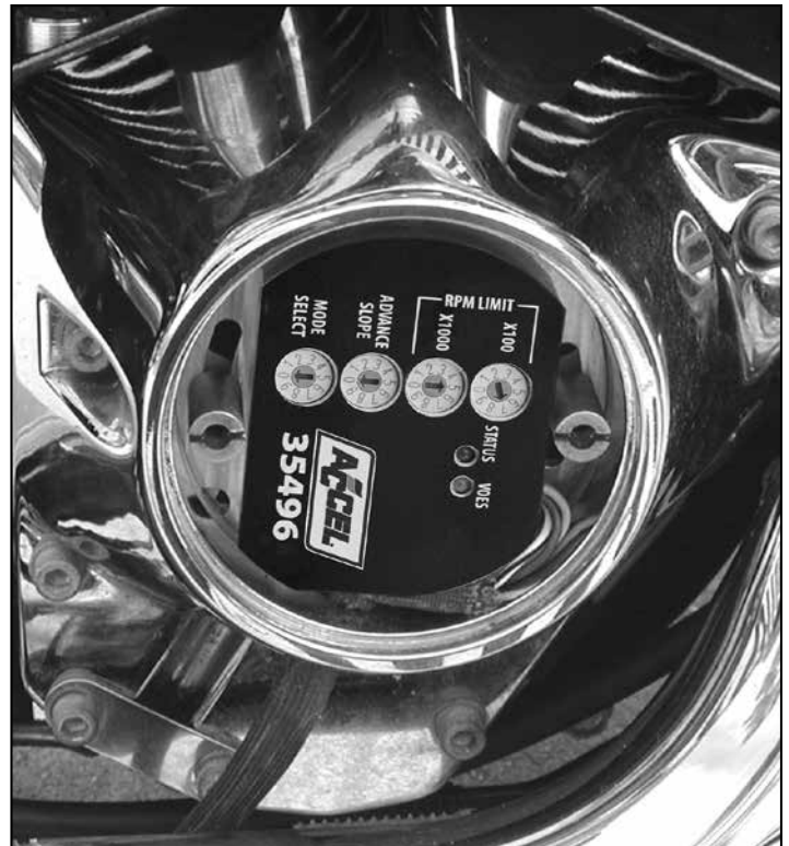
Figure 3A - Finished Big-Twin® Installation
