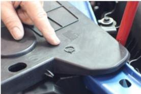
2. The next spot to grab some clearance will be at the headlight bracket bolted to the radiator support rail and the criss cross bracket of the rail itself. These two areas will need to be sanded down about a quarter inch at both ends of the header area. See pictures below.
