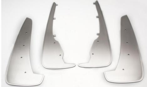
PARTS INCLUDED: 4-Mud Guards 12-1" Washer Head Screws 12-Clip Nuts
