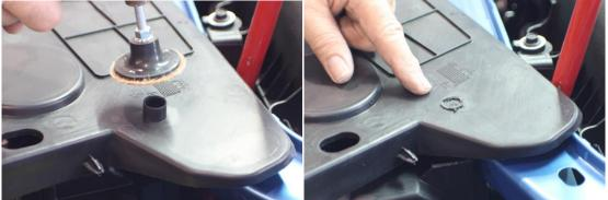
2. The next spot to grab some clearance will be at the headlight bracket bolted to the radiator support rail and the criss cross bracket of the rail itself. These two areas will need to be sanded down about a quarter inch at both ends of the header area. See pictures below.
