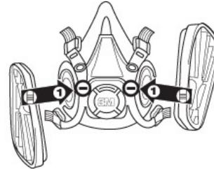
2. Turn adapter ¼ turn clockwise to stop. To remove adapter, turn ¼ turn counter-clockwise.
