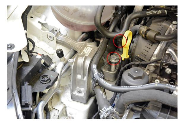
**Step 28** – Remove the factory Engine Mount.
