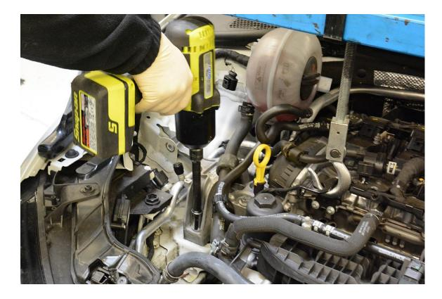
**Step 23** – Using a 16mm swivel socket, remove the 4 bolts securing the Transmission Mount to the frame rail.
