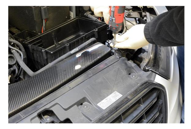
**Step 6** – Remove the factory Front Air Duct.
