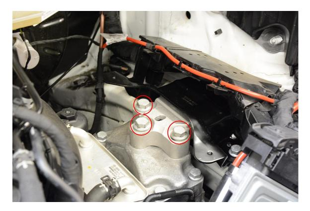
**Step 31** – Properly torque the hardware for the Engine Mount and Transmission Mount. Factory torque specs for new hardware are below. If you wish to reuse the OEM hardware, they can be torqued to the *initial torque value* if installed with Blue Loctite.
