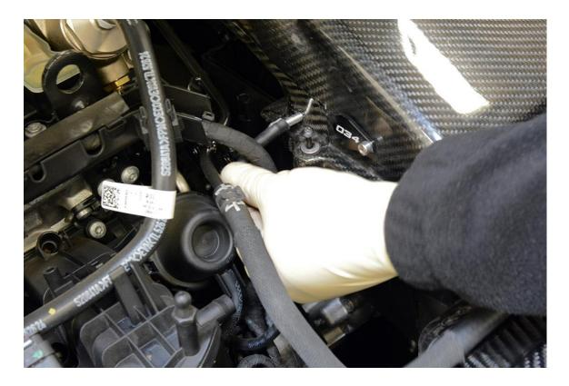
**Step 5** – Remove the two T25 Torx screws securing the factory Front Air Duct.
