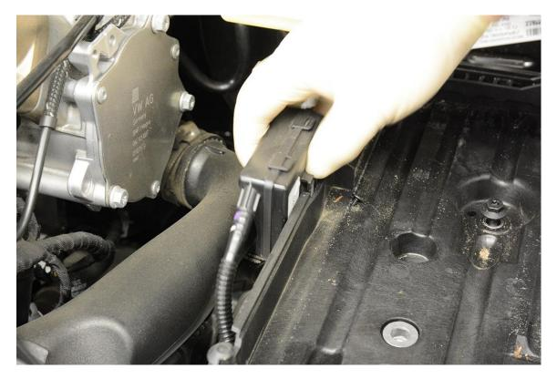
**Step 12** – Unclip the factory ECU from the plastic holder, and move it out of the way to access the fuse box.
