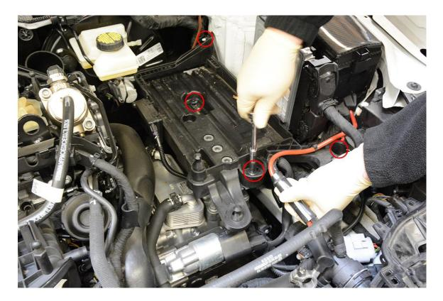
**Step 11** – Unclip the plastic case/harness attached to the battery tray.
