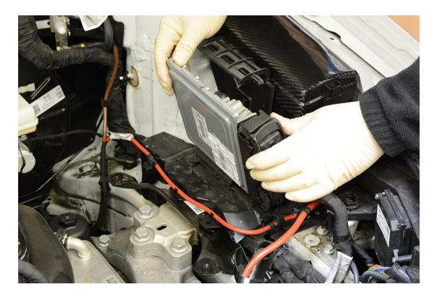
**Step 13** – Using a 10mm socket, remove the two nuts securing the ECU holder to the fuse box. Remove the plastic ECU holder.
