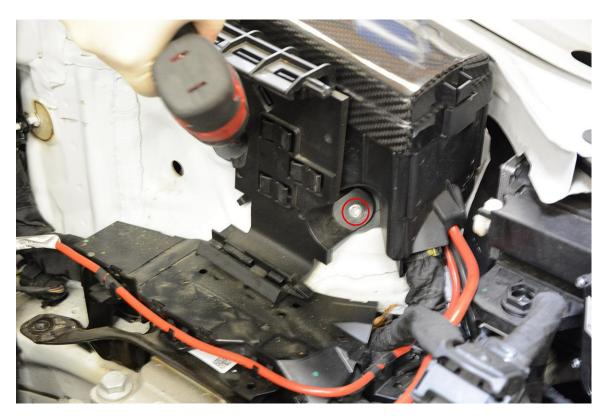
**Step 14** – Lift the factory wiring harness cover up firmly to gain access to the four bolts securing the Transmission Mount to the frame rail.
