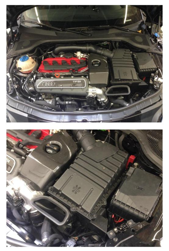
**Step 2** – Remove the carbon piece over the valve cover, around the oil cap. Remove the air duct to the airbox as well. Unclamp the bypass hose and the intake flex hose.
