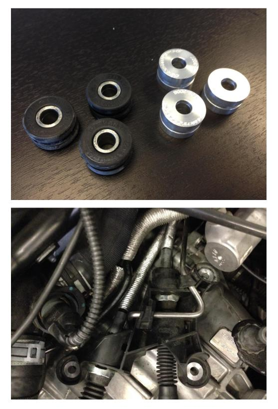
**Step 6** – Install the top half of the aluminum bushings, and reuse the stock mounting bolts. Tighten to 20 Nm.
