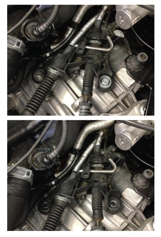
**Step 5** – Remove OEM rubber bushings and replace with 034Motorsport Billet Aluminum pieces. The larger part goes on the bottom, mating to the transmission.
