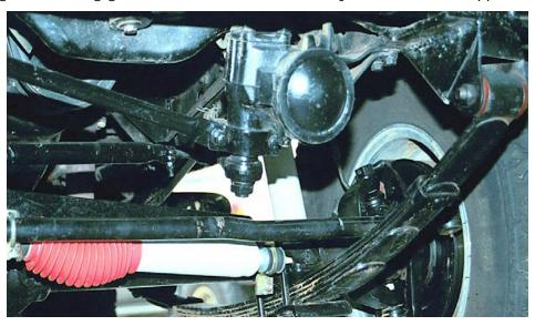
**Step 1** Remove the bolt from the coupler that couples the intermediate shaft to the input shaft of the steering gearbox.
