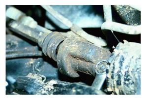
**Step 2** Remove the power steering hoses from the steering gearbox.
