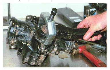
Step 8 Remove the mount bolts that retain the gearbox in the chassis. On some vehicles you must remove the steering gearbox with the mount brackets attached and then remove the mount brackets once the gearbox is on the workbench. As you are removing the gearbox, you can then disconnect the intermediate shaft coupler from the input shaft of the gearbox. You might have to use a mallet and tap on the coupler to get it to slide off of the input shaft.
